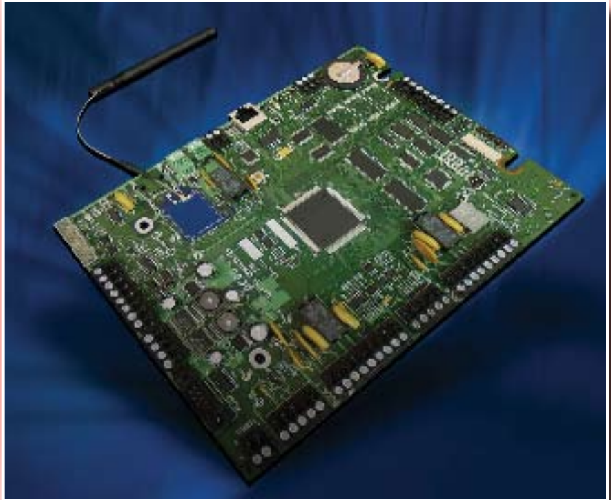
The Fault Tolerant controllers from PCSC use a redundancy methodology that allows any master controller on the system to step up and take the place of any failing master controller on the system.
